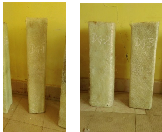
Figure 5. Double layered GFRP wrapped Columns
