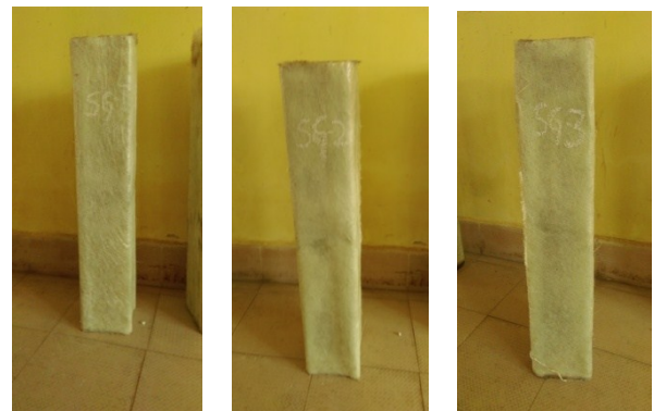
Figure 4. Single layered GFRP wrapped Columns
