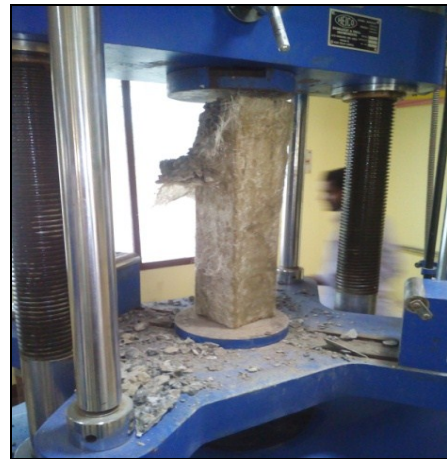
Figure 9. Failure of Single layered GFRP Wrapped Column
