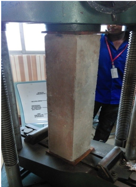
Figure 6. Axial Compressive load on Control Column
