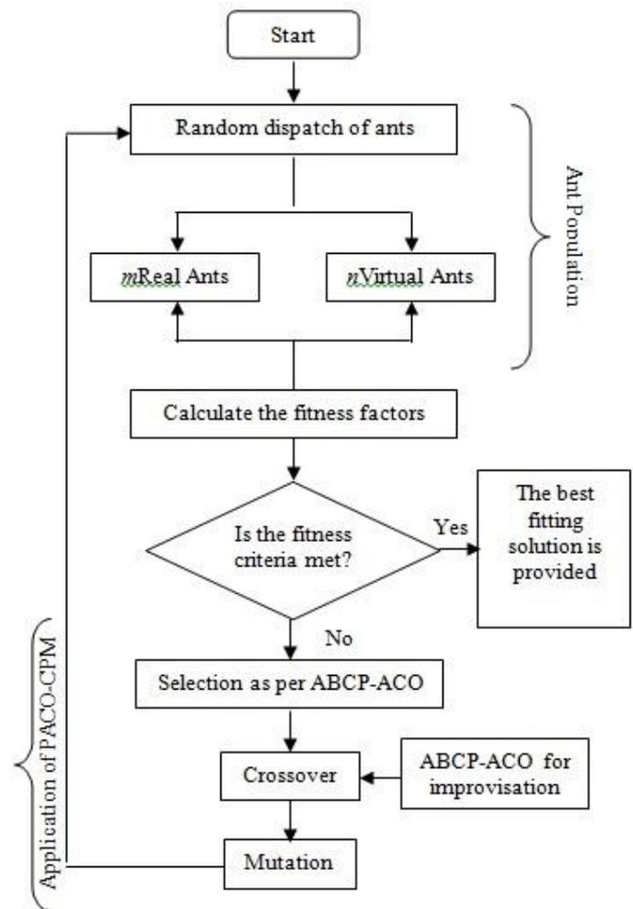
**Figure 1:** Evolutionary Workflow of Genetic Algorithm for Hybrid ABCP-ACO Algorithm
