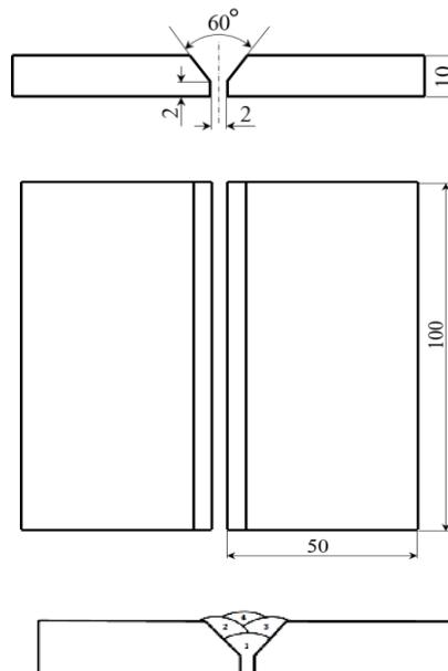
**Figure 1:** Schematic illustration of the workpiece of this experiment.
