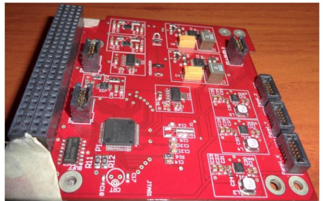
Figure 10: Principal board implemented of version 1 of Critical Design of Power Module in CubeSat Colombia 1.
