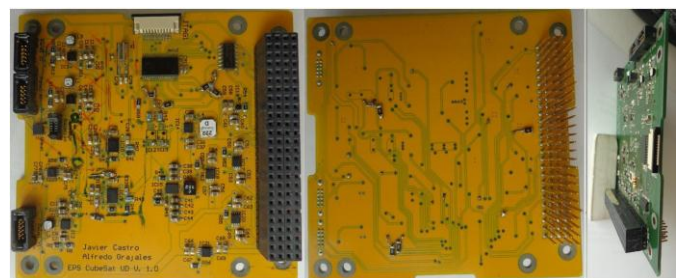
Figure 8: Implementation of version 1 of Critical Design of Power Module in CubeSat Colombia 1.
