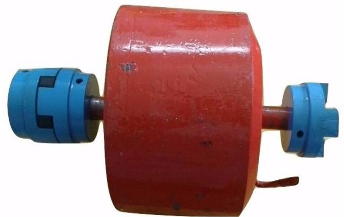
Figure 5: Cross Section of Magneto Rheological Fluid Clutch and its Assembly with Couplings
