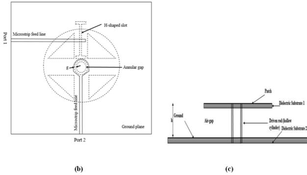
(b) Bottom-view (c) Side-view of an antenna
