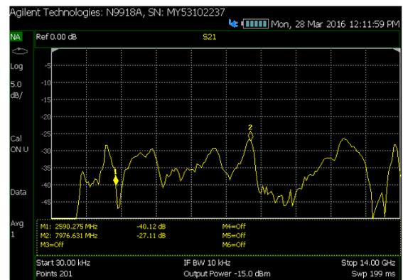
**Figure 7:** Measured  $S_{21}$  of the proposed antenna
