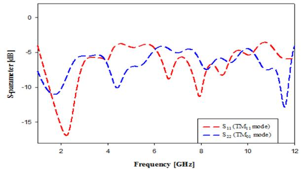
Figure 2: Simulated reflection coefficient of proposed antenna structure
