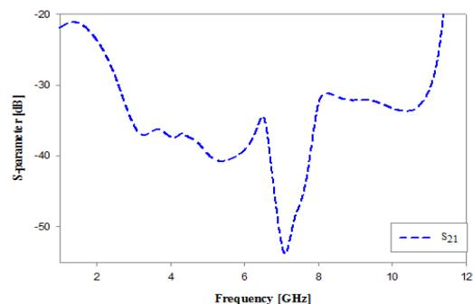
Figure 3: Simulated  $S_{21}$  parameter of proposed antenna structure
