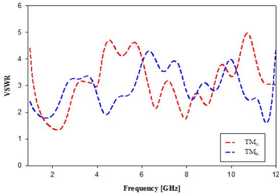
**Figure 4:** Simulated VSWR of proposed antenna structure
