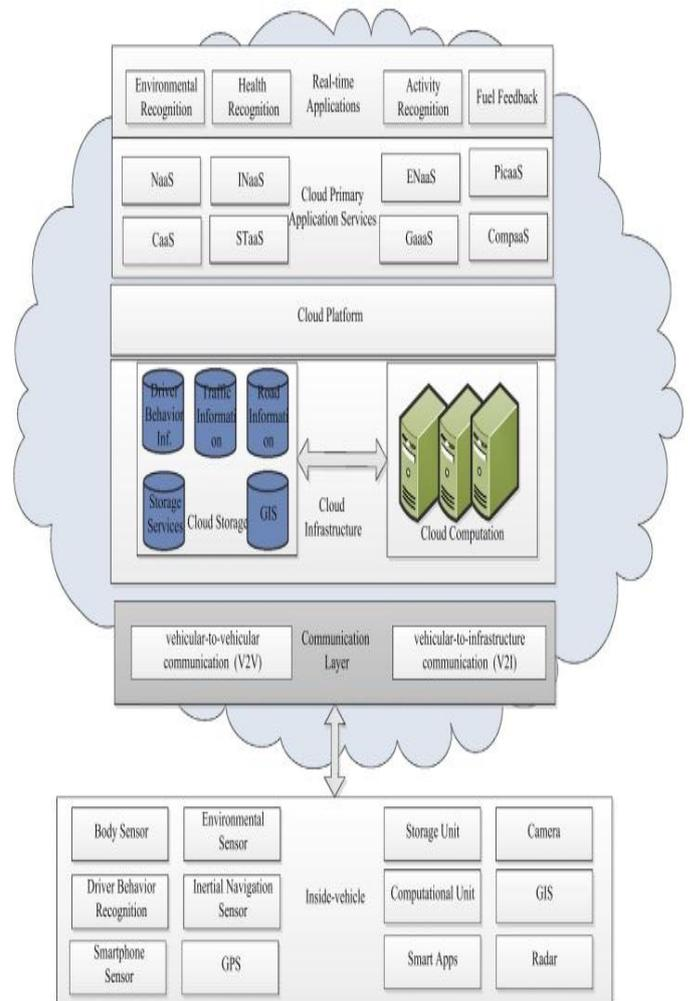
**Figure 1:** Vehicular Cloud Computing Architecture [16][15].
