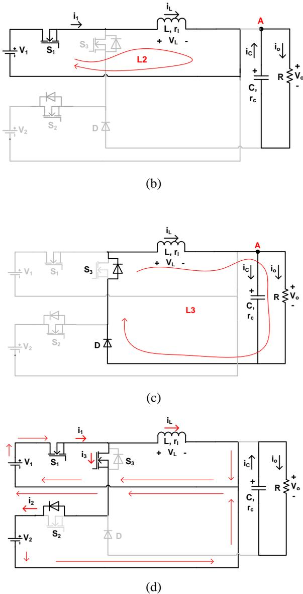
**Figure 2:** Operating circuits of the proposed MIC ( $V_1 > V_2$ ): (a) State 1. Charging of  $L$  by  $V_2$ , (b) State 2. Charging of  $L$  by  $V_1$ , (c) State 3. Charging of  $C$  by  $L$ , (d) State 4. Charging of  $V_2$  and  $L$  by  $V_1$
