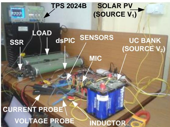
**Figure 7.** Laboratory setup of MIC
