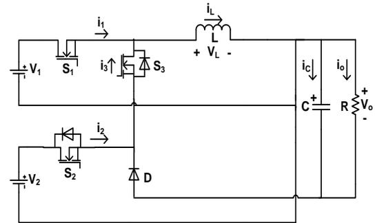
**Figure 1:** Circuit diagram of the proposed MIC
