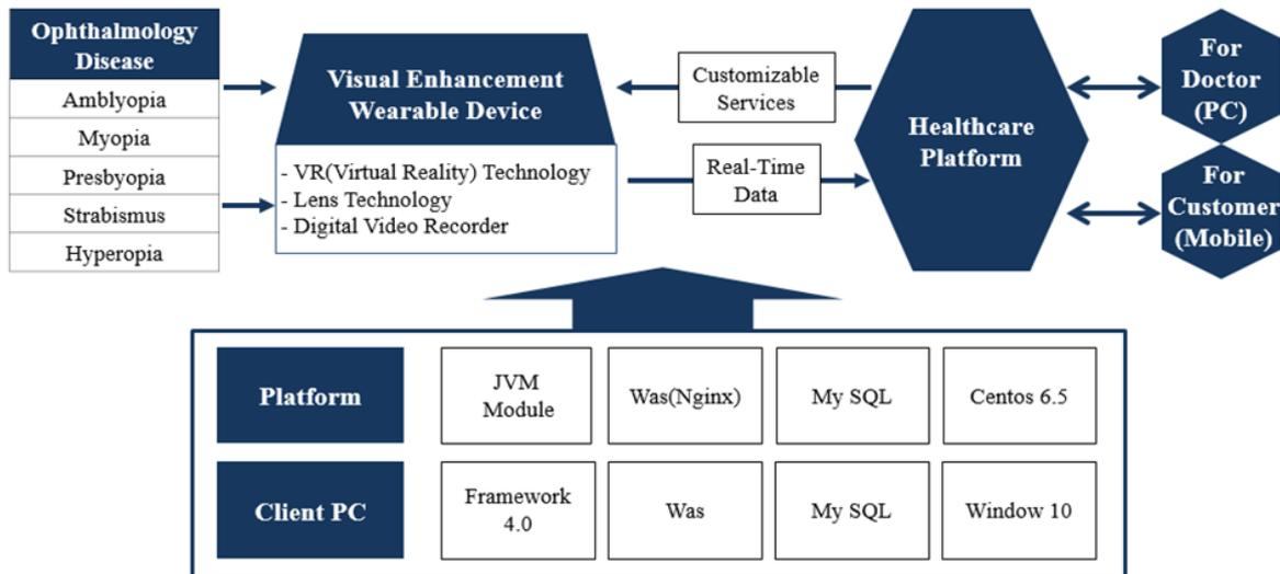
**Figure 2:** Overall Configuration of a System Having an Optometric Image Analyzer Based on Multi-Modal Sensing Data
