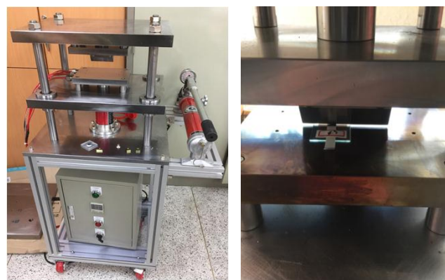
Figure 3: The ACF bonding press
