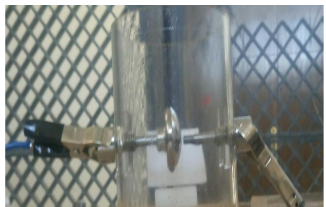
(b) Pin-hemisphere test Cell with a gap distance 1.66 mm.
