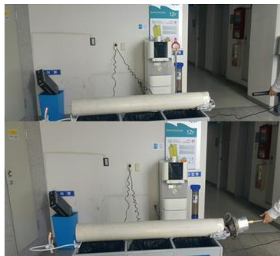
Figure 2: Sound Fire Extinguisher Experimental Scene
