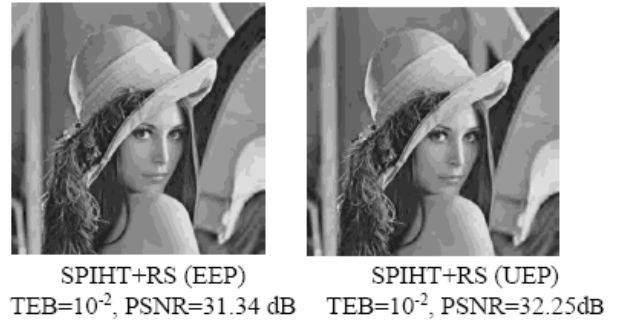
Figure 6: Recieved image (Lena) with EEP and UEP protection transmitted in BSC channel (CR = 0.25 bpp).
