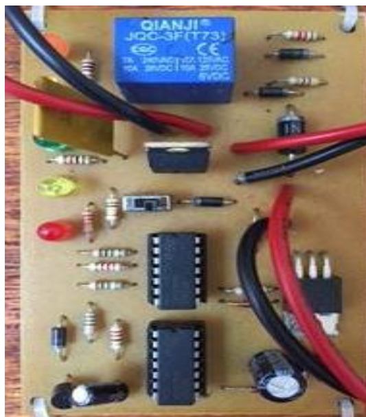
Figure 3: Solar charge controller PCB board
