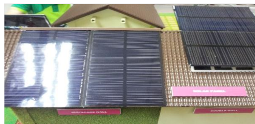
Figure 4: Solar panel and solar tracker attached on the roof of house model
