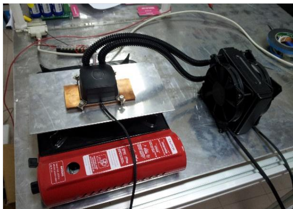
Figure 6: Thermal electric generator module
