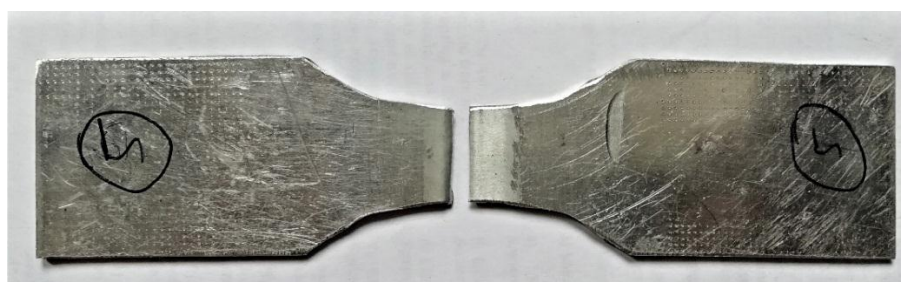
Figure 6. specimen after tensile test
