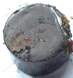
Figure 2.2. Copper coated sample with interlayer
