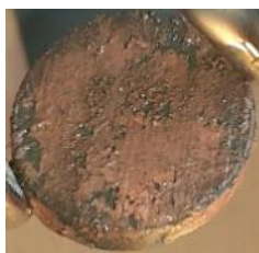
Figure 2.3. Copper coating with phosphate degreasing
