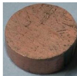
Figure 2.4. Copper coating with pyrophosphate etching
