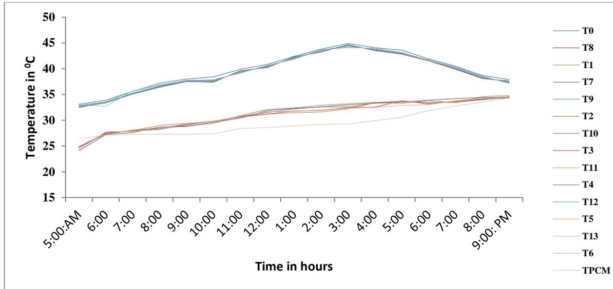
Figure 9. Variation of inside and outside test room temperature w.r.t PCM during discharging.
