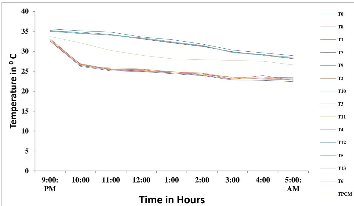
**Figure 6.** Variation of inside and outside test room temperature w.r.t PCM during charging.
