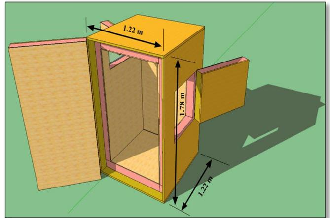
**Figure 1.** Test room construction and dimensions
