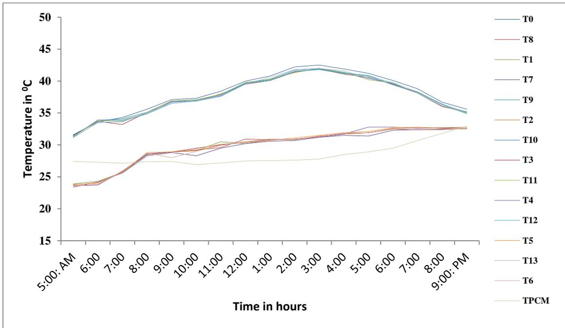
Figure 7. Variation of inside and outside test room temperature w.r.t PCM during discharging.
