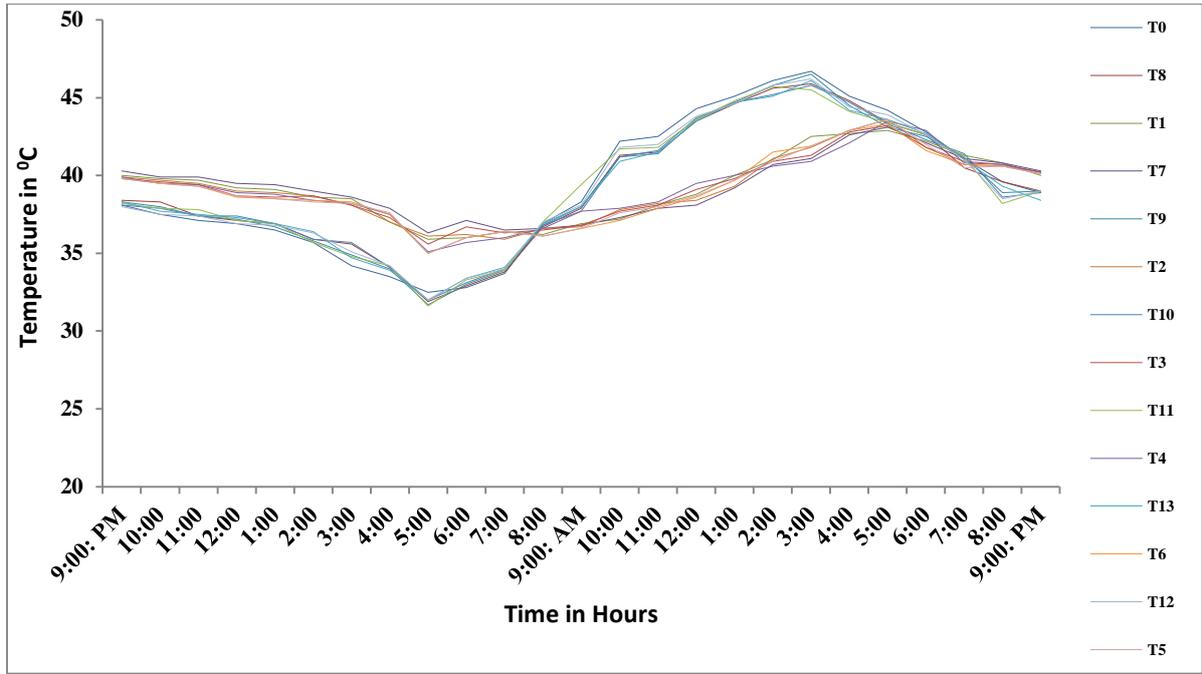
**Figure. 5.** Temperature profiles of ambient air, inside test room air, outer test room surfaces and inner test room surfaces.
