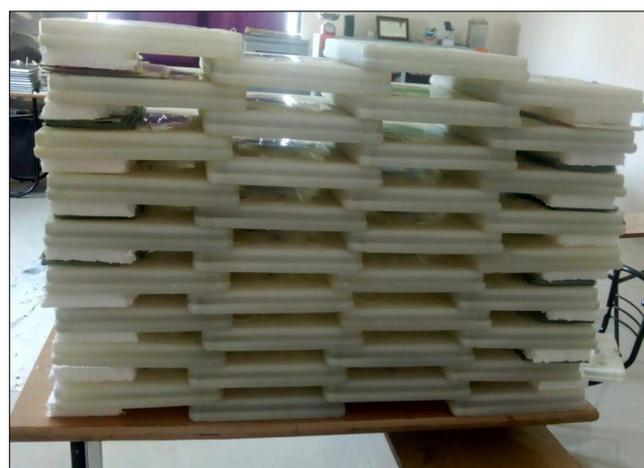
**Figure 4.** Arrangement of PCM Panels.
