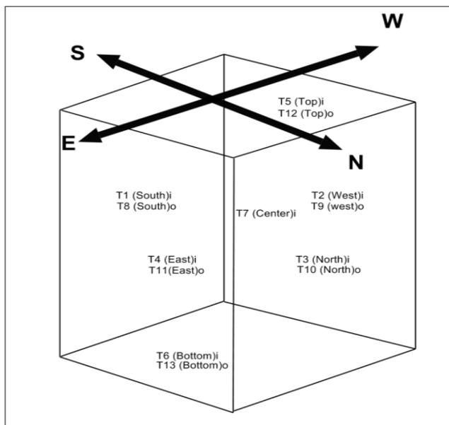
**Figure 3.** Schematic description of the thermocouples installed in the test room.
