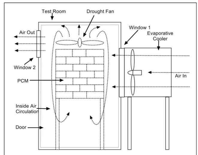
**Figure 2.** Schematic description of the thermal management system.
