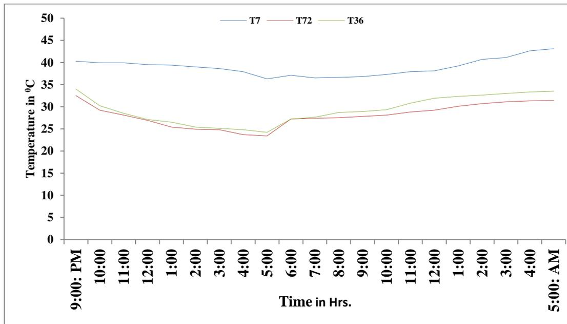
Figure 10. Comparative analysis of inside test room temperature variation with and without TMS
