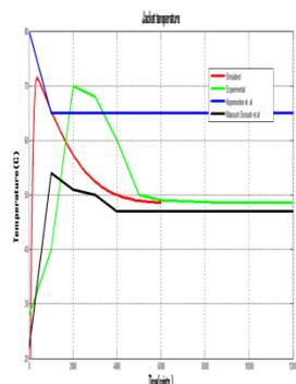
Servo operation of the controller scheme for the reactor temperature
