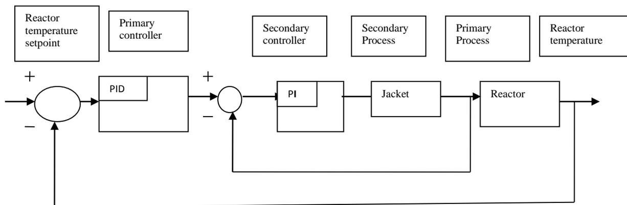
**Figure 4.** Block diagram of closed loop cascade control scheme for PVC resin process
