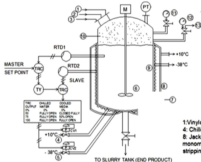
1. vinylchloride monomer, 2. Pure water, 3. Catalyst and initiator, 4. Chilled water, 5. Cooled media, 6. Agitator, 7. Limbed coil, 8. Jacket, 9. Glass lined surface, 10. Unreacted vinyl chloride monomer, 11. Pressure gauge, 12. Vacuum gauge, 13. Vacuum stripping
