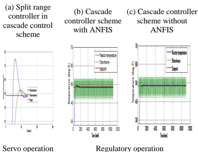
**Figure 9.** Closed loop cascade controller response of PVC resin process
