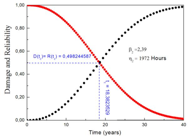
**Figure 9:** The Reliability (survival) function and The Damage factors as a function of time with  $\beta_2 = 2.39$  and  $\eta_2 = 1972$  Hours .
