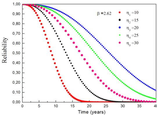
**Figure 4:** The Reliability (survival) function  $R(t)$  as a function of time for different values of  $\eta$  with  $\beta = 2.62$
