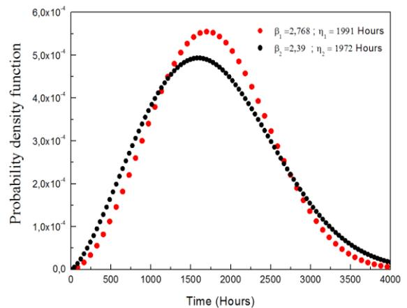
**Figure 7:** The Weibull Probability Density Function  $F^{PDF}(t)$  as a function of time.  $\beta_1 = 2.768$  and  $\eta_1 = 1991$  Hours (red scatter).
