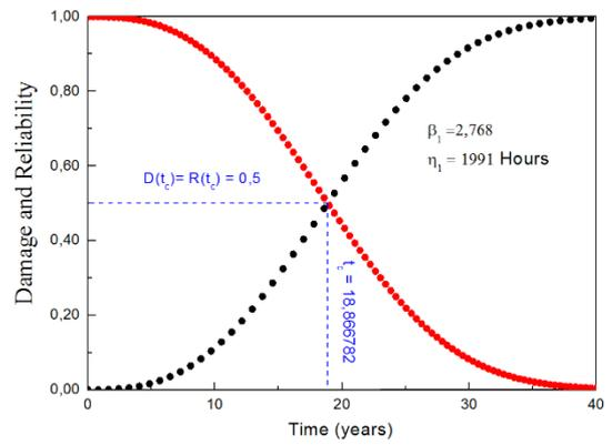
**Figure 8:** The Reliability (survival) function and The Damage factors as a function of time with  $\beta_1 = 2.768$  and  $\eta_1 = 1991$  Hours .
