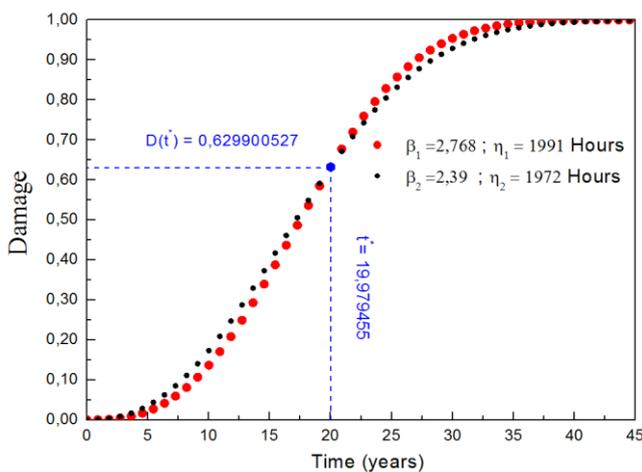
**Figure 2:** The corrosion factor  $D(t)$  as a function of time.
