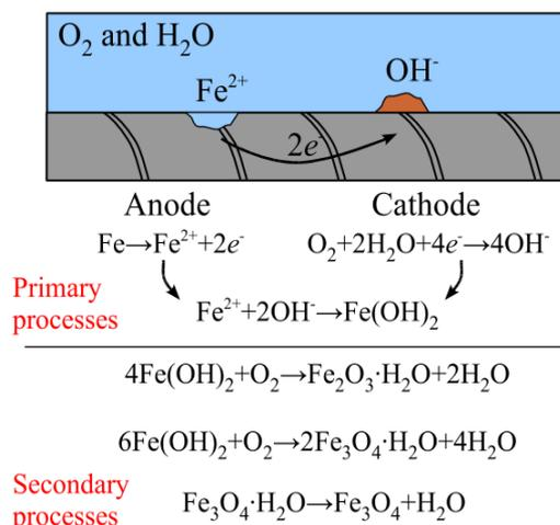
Figure 1: Electrochemical corrosion mechanism of Iron [21]
