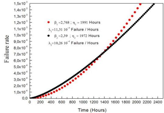
**Figure 6:** The Weibull Failure Rate Function (FRF) as a function of time with  $\beta_1 = 2.768$  and  $\eta_1 = 1991$  Hours (red scatter).
