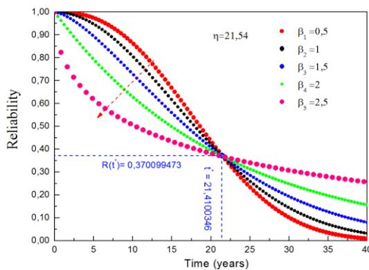
**Figure 5:** The Reliability (survival) function  $R(t)$  as a function of time for different values of  $\beta$  with  $\eta = 21.54$
