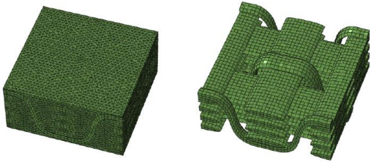
Figure 5. “Rough” (29 thousand nodes) KE model of RVE.
