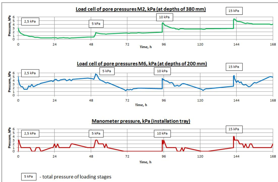
**Figure 9:** Pore pressure graphs for the first 7 days of the experiment.
