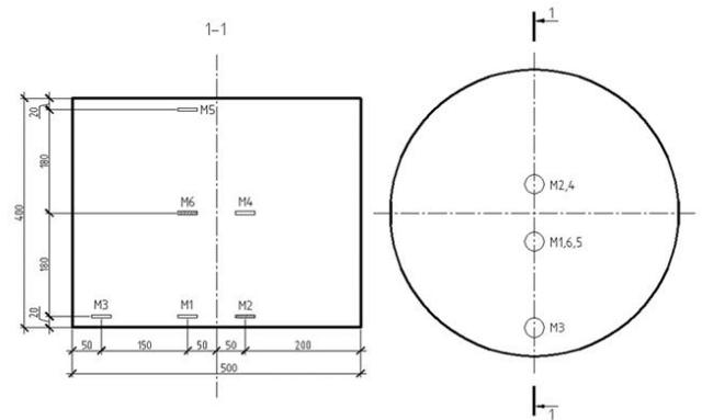
**Figure 3:** Scheme of the load cells in the soil sample. M 1,3,4,5 for load cells of general pressures. M 2,6 for load cells of pore pressures.
