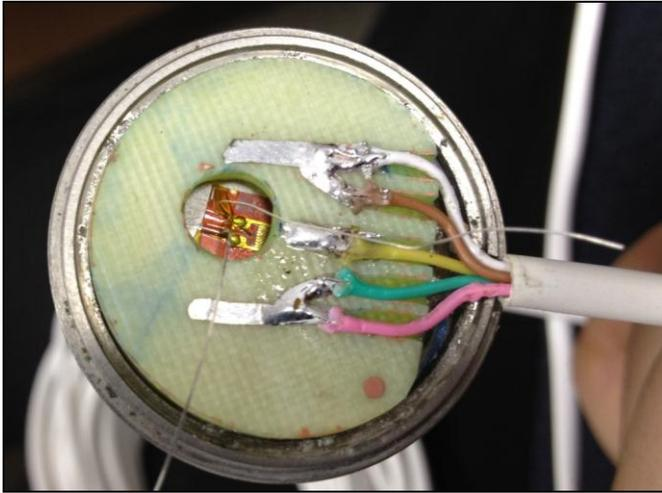
**Figure 5:** The upgraded load cell.
