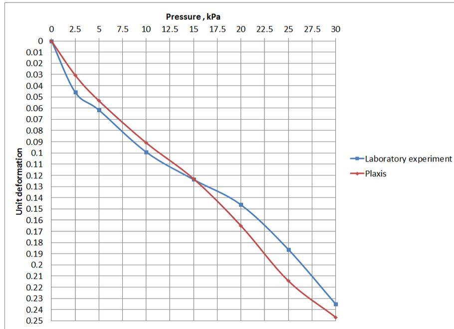
**Figure 8:** Unit deformation-pressure diagram.
