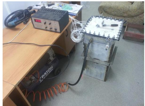
**Figure 4:** An aerostatic tank with air compressor.
