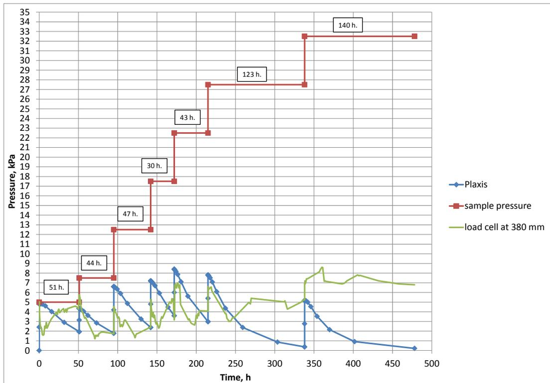
**Figure 11:** Graph of the excessive pore pressure against sample pressure at depths of 380 mm.
