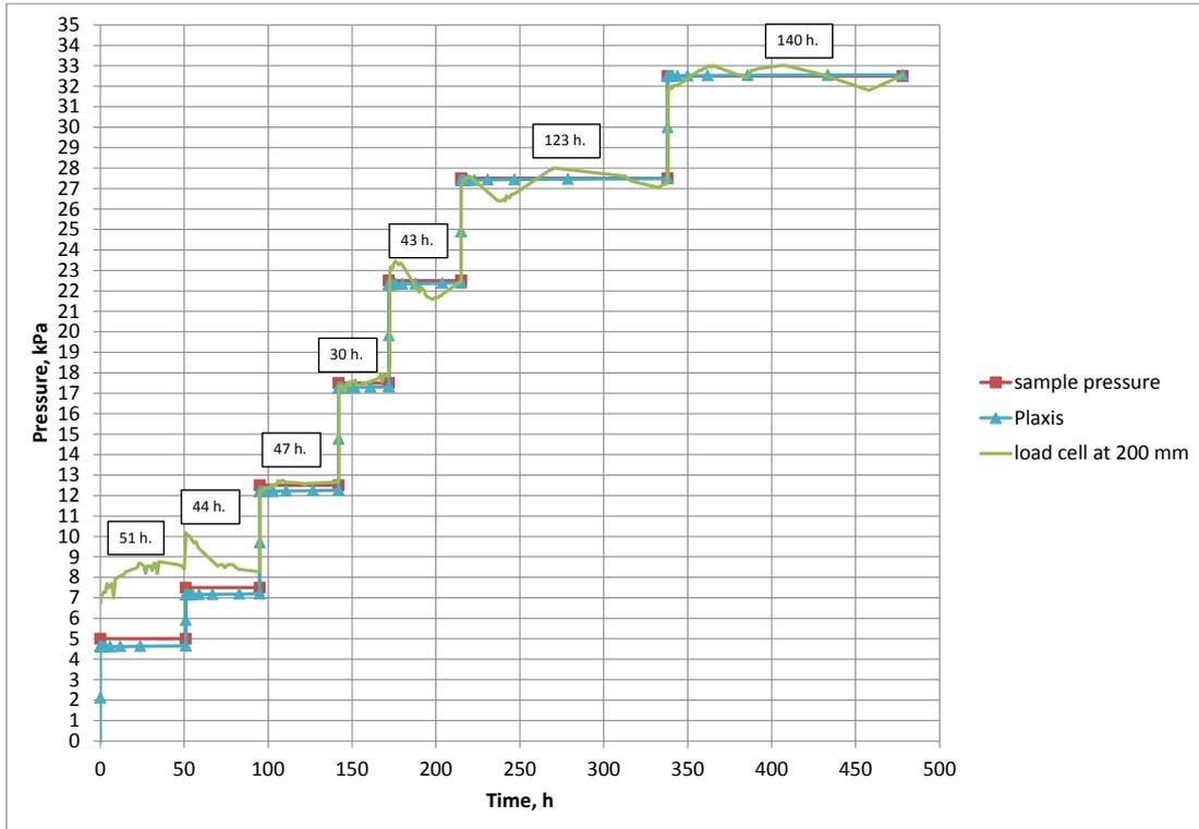
**Figure 10:** Graph of the stresses in soil against the sample pressure at depths of 200 mm.
