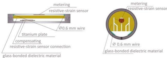
**Figure 6:** The scheme of upgraded load cell.
