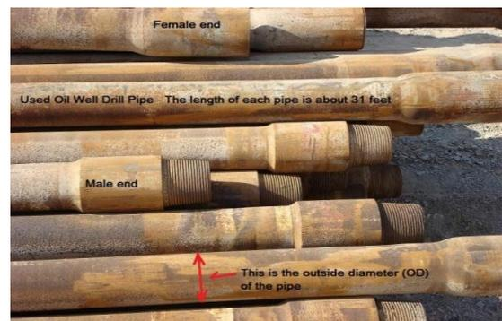
**Figure 3.** The oil drilling pipe body
