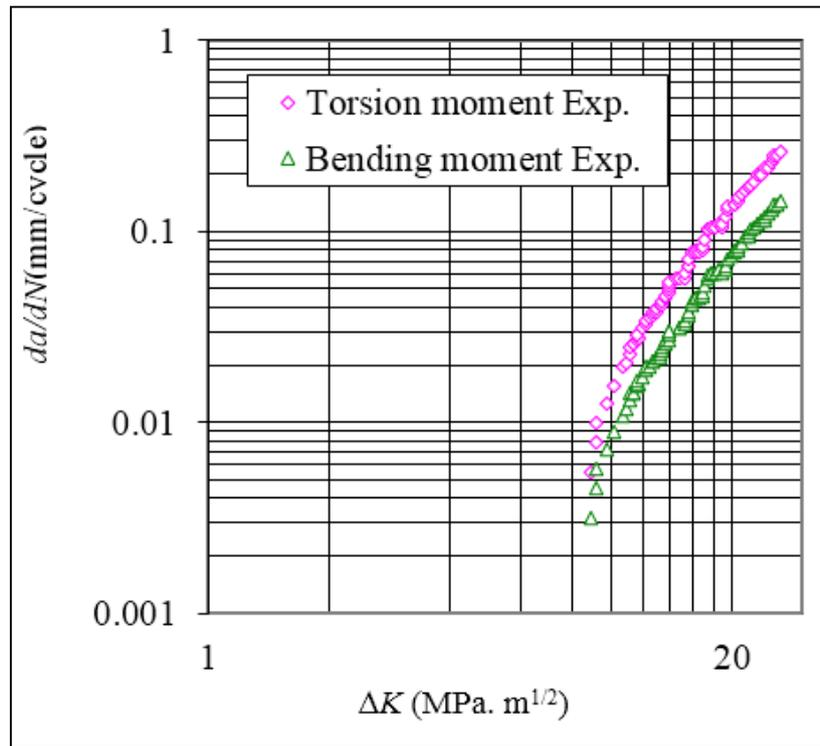
Figure 10. FCGR comparison between bending and torsion moment
