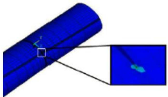
**Figure 7.** Crack meshes under torsion moment
