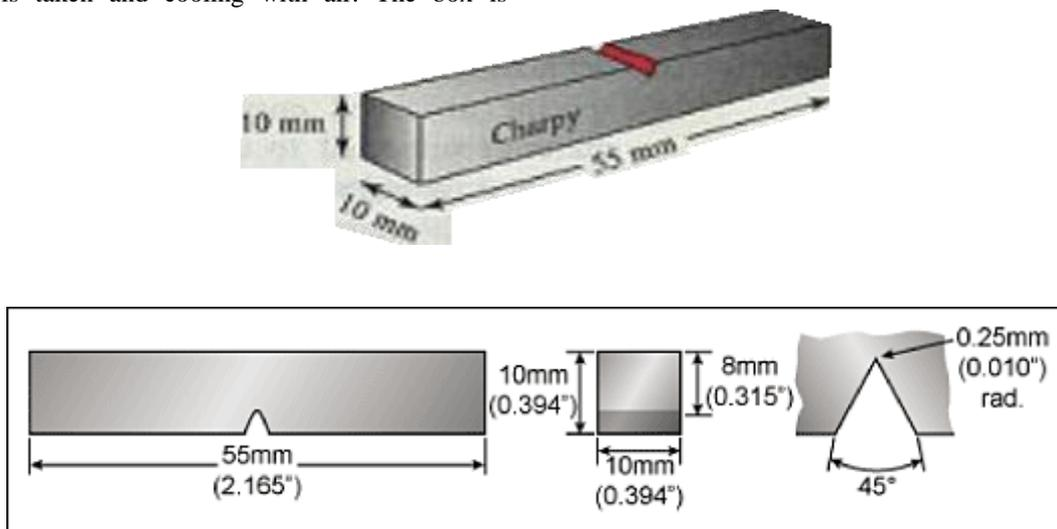
**Figure 2.** Spesimens of impact testing standar ASTM E 23-56T (Suherman.W, 1987).
