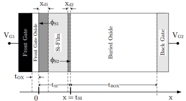
Figure 2. Metal-Oxide-Semiconductor-Oxide-Semiconductor structure.
