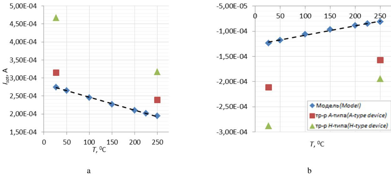
Figure 4. Temperature dependencies of saturation currents  $I_{sat}$  for: a – NMOS transistor; b – PMOS-transistor.
