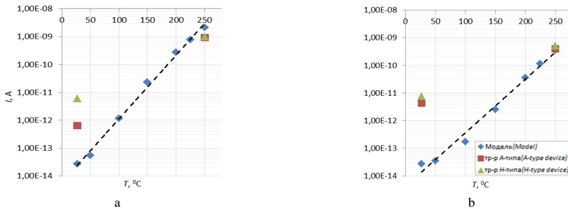
**Figure 5.** Temperature dependencies of leakage currents  $I$  for: a – NMOS transistor; b – PMOS-transistor.
