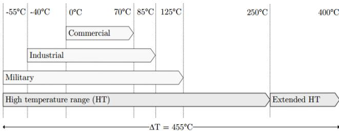
Figure 1. Operating temperature ranges according to their specific application.
