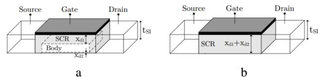
Figure 3. a – partially depleted transistor; b – fully depleted transistor.
