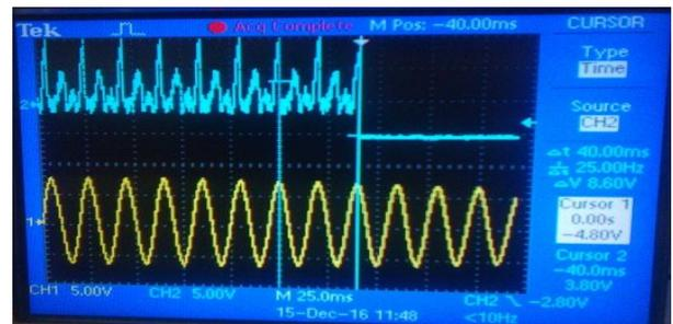
**Figure 6.** Voltage dip to 173 volts; Relay response time: 40 ms.
