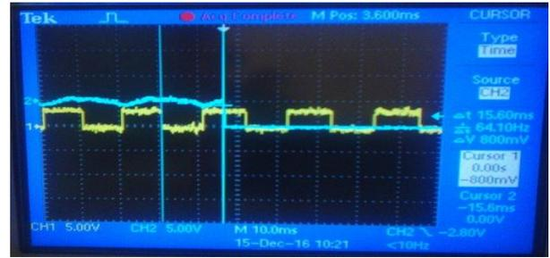
**Figure 4.** Frequency dip to 47 Hz; Relay Response Time 15.60 ms (Yellow: Frequency; Blue: Relay)
