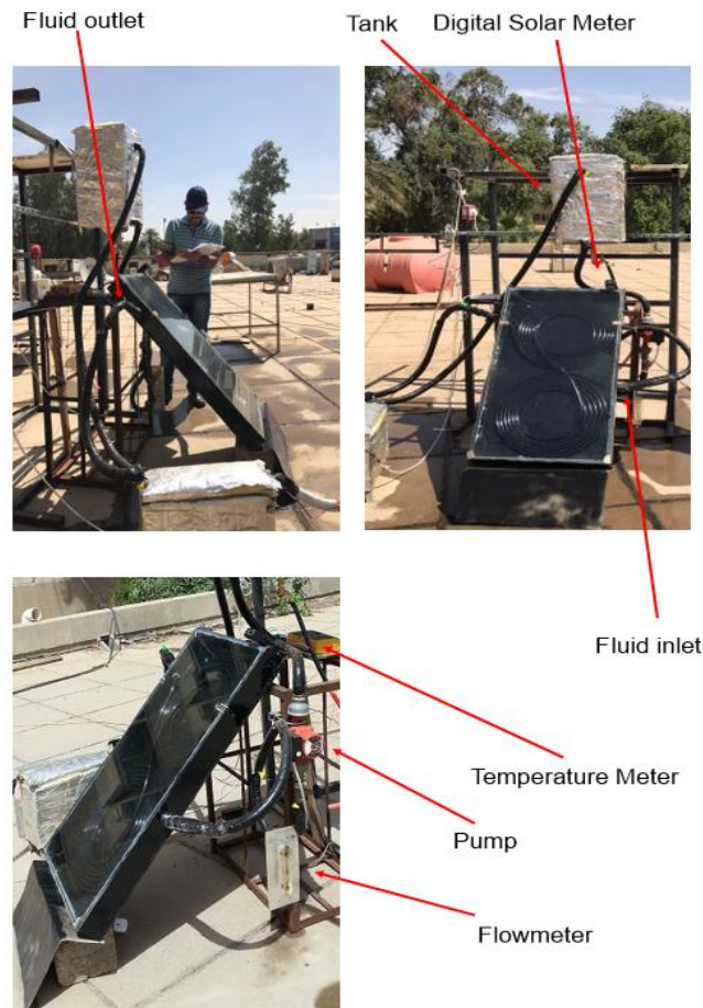
Figure (2): Experimental set-up of flat plate solar collector.
