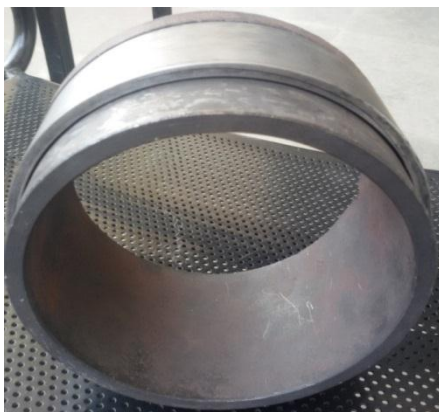
Figure 8a: ISSFD Ring on a hollow mandrel
