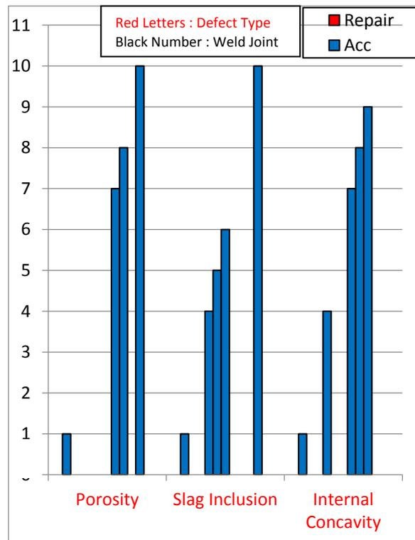
It can be seen from the test results of weld joint after re-welding, the welding results are indeed still have a welding defect. This is because the final result of weld joint is repairs from failed welded joint material so that it does not get maximum results but the test results shows weld joint pass the acceptance standard criteria and may continue to the next work process.
