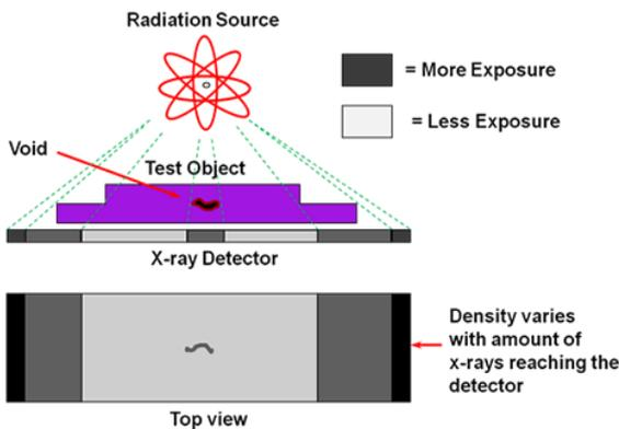
Figure 5. Radiography Test Method<sup>[14]</sup>
