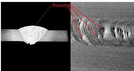
Figure 1. Weld Porosity on Pipe<sup>[9]</sup>
