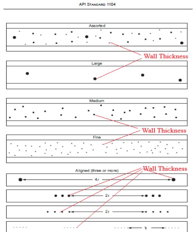
Figure 2. Maksimum distribusi of Gas Pockets : WallThickness ( $t$ ) less than/equal to 12.7 mm <sup>[8]</sup>
