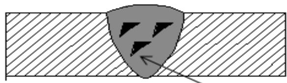
Figure 3. Slag Inclusion Illustration<sup>[10]</sup>
