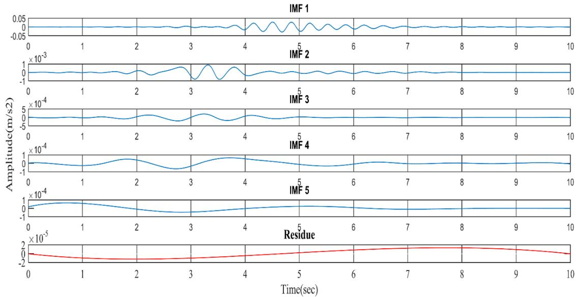
**Figure 5:** Filtered signal response of the third-floor inherent mode functions.
