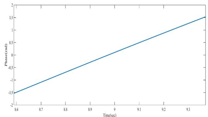
**Figure 7:** Phase curve of the first IMF of the third-floor refined response signal
