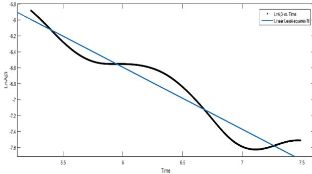
**Figure 8:** Least squares fit to the logarithmic instantaneous amplitude of the first IMF of the third-floor refined response signal.
