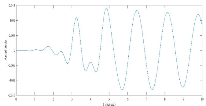
**Figure 4:** Refined response for the third floor in free vibration mode in the range of  $0.3 < \omega < 1.8$ .
