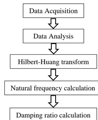
**Figure 1:** A diagram of the phases of the system's dynamic characteristic determination process using HHT.
