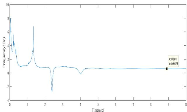
**Figure 6:** The instantaneous frequency of the first intrinsic mode function of the third-floor refined signal response.
