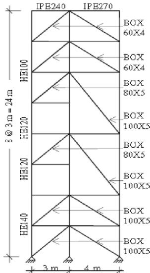
**Figure 2:** Characteristics of the two-dimensional sections of the structure with eight degree of freedom.
