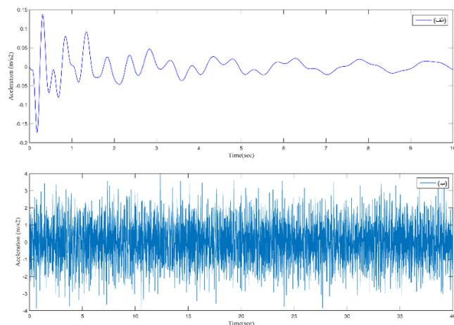
**Figure 3:** Output of the acceleration of the third floor (a) free vibration (b) forced vibration resulted from random load on the first floor.
