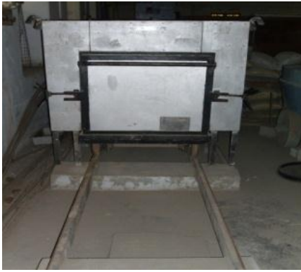
Fig. 2 (b) RC beam specimens in to the heating chamber
