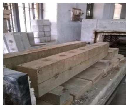
Fig. 2 (a) RC beam specimens before heating
