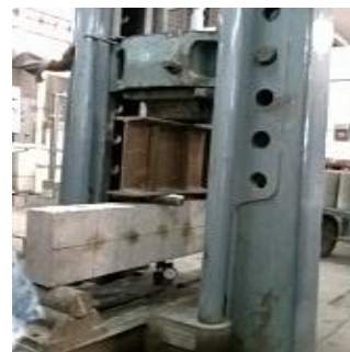
Fig. 7 RC repaired beam in UTM under two point loading
