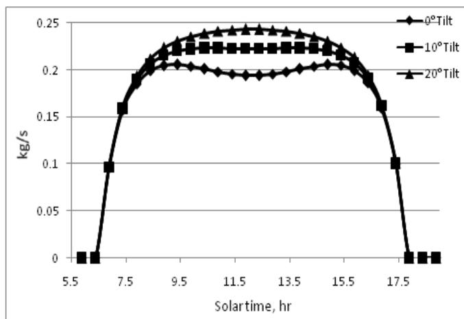
**Figure 10.** Hourly rate of fresh water production for the month of March at 0°, 10°, 20° tilt angles.
