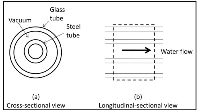
**Figure 3.** Finite control volume used for the development of the governing equations.
