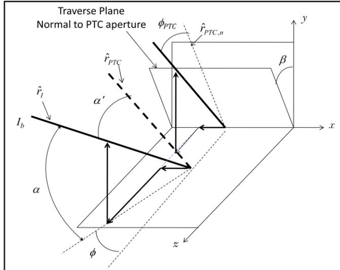
**Figure 2.** Definitions of incidence, tilt, rotation angles and unit vectors.
