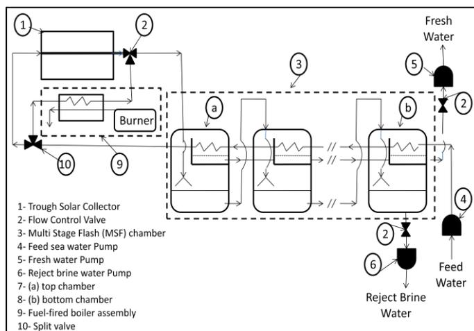
Figure 1. Solar-fuel desalination scheme.
