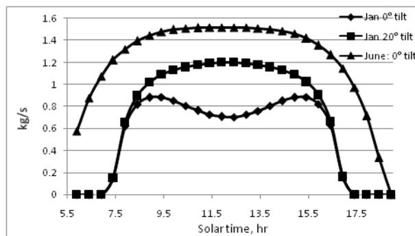
Figure 5. Hourly rate of seawater flowing through the PTC.
