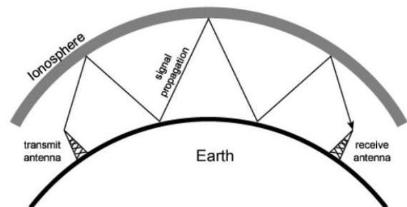
Fig 1. HF Radio Wave Propagation
