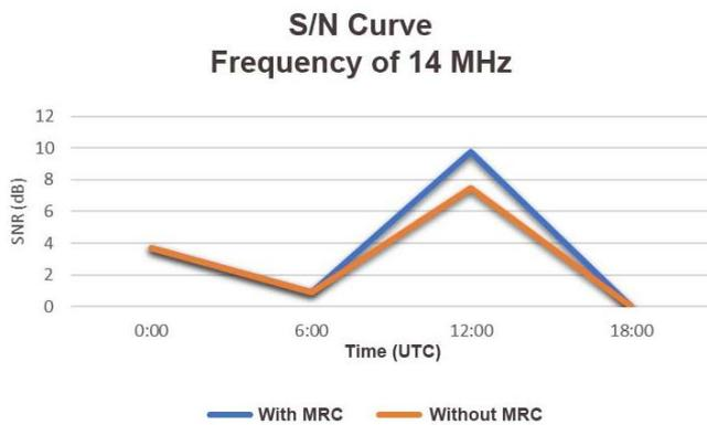
Fig 4. Curve of  $\frac{S}{N}$  14 MHz Frequency Calculation
