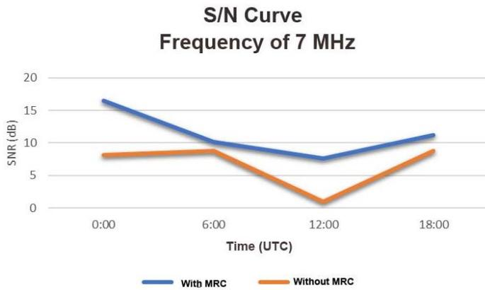
Fig 3. Curve of  $\frac{S}{N}$  7 MHz Frequency Calculation
