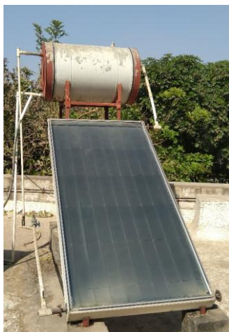
Fig. 3 Solar water heater experimental setup
