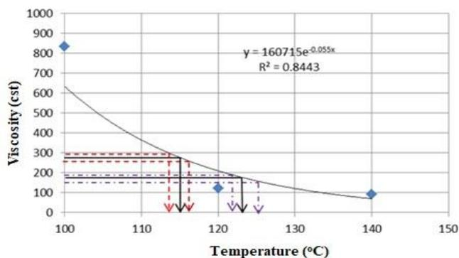
**Figure 3.** Relationship of Viscosity and Temperature
