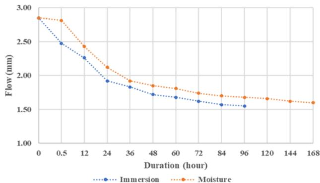
Figure 5. Effect of Immersion and Moisture on Flow
