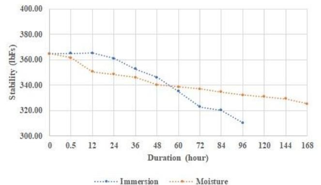
Figure 4. Effect of Immersion and Moisture on Stability
