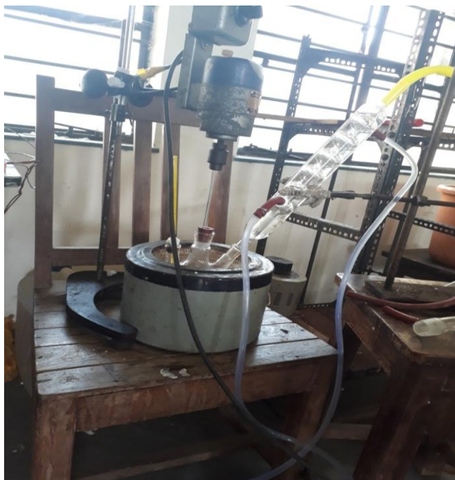
Fig.3. Biodiesel Batch Reactor
