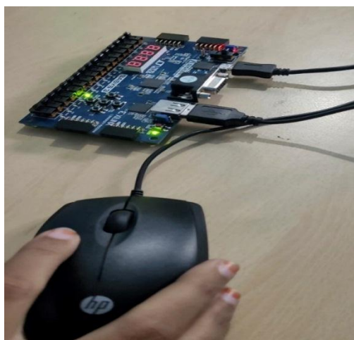
Figure 3.2 Mouse interface with Artix7 FPGA board for left click
