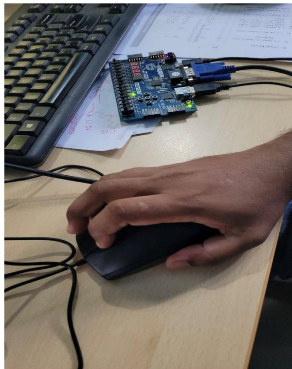
Figure 3.4: Mouse interface with Artix7 FPGA board for scroll
