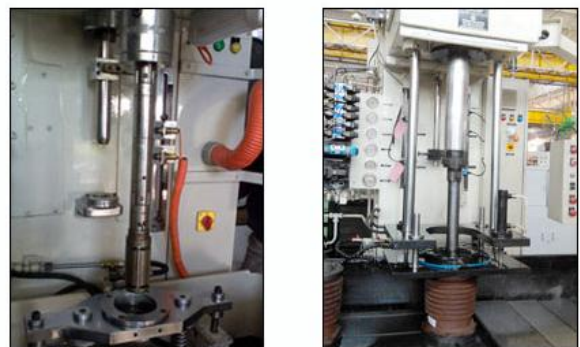
Fig. 1: Honing Head with Tooling (Honda Ltd. Gurgaon)
