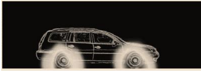
Figure 2: Propagation of tyre noise of an automobile at frequency of 600 Hz
