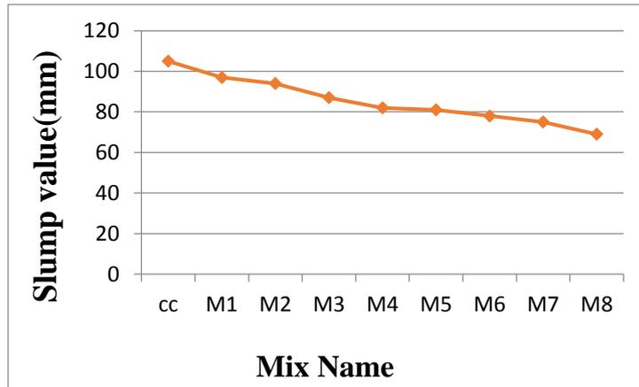
Fig.5.1 Slump values for various mix
