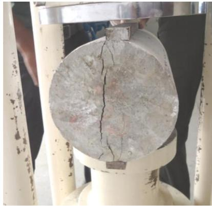
**Fig. 7.** Compression strength of concrete (without fibre)
