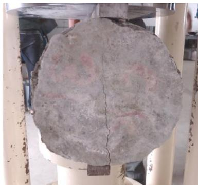
**Fig. 8.** Compression strength of reinforced concrete
