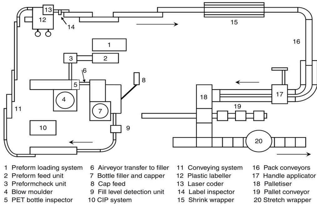
**Figure 2:** A compact PET bottle filling line.
