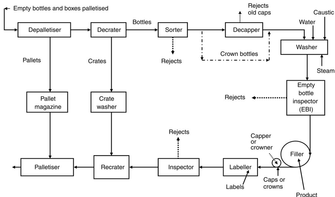
**Figure 1:** Typical returnable glass bottle filling line.
