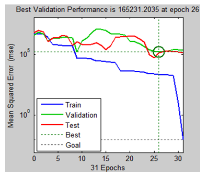
Fig 8 Variation of Mean Squared Error (MSE) With Number of Epochs for Flexural Strength
