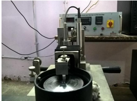
Figure 3: Pin on Disk Wear Testing apparatus
