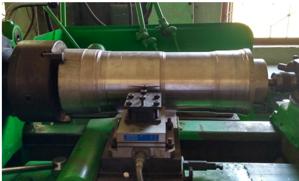
Fig 3:- Image of rolled aluminium and 3-componenet Kistler dynamometer mounted on lathe
