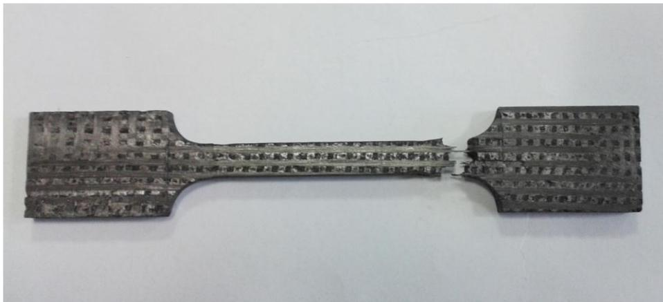
**Figure 5:** 3-D sample Tensile failure
