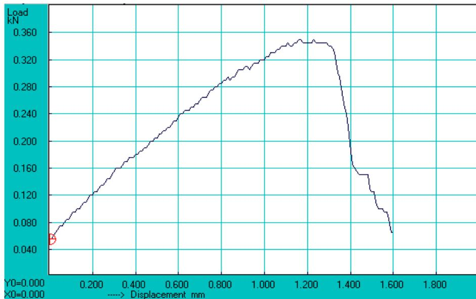
**Graph 5:** 3-D sample 1,1,4 tested for Flexural strength in X direction
