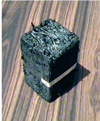
**Figure. 3:** 3-D Carbon fibre preform
