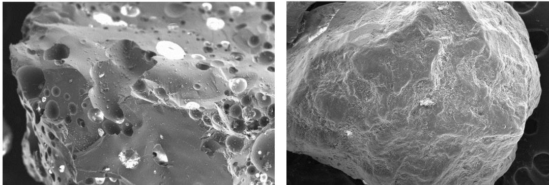
**Fig 2:** Comparison of particle morphology (a) River sand (b) GBS
