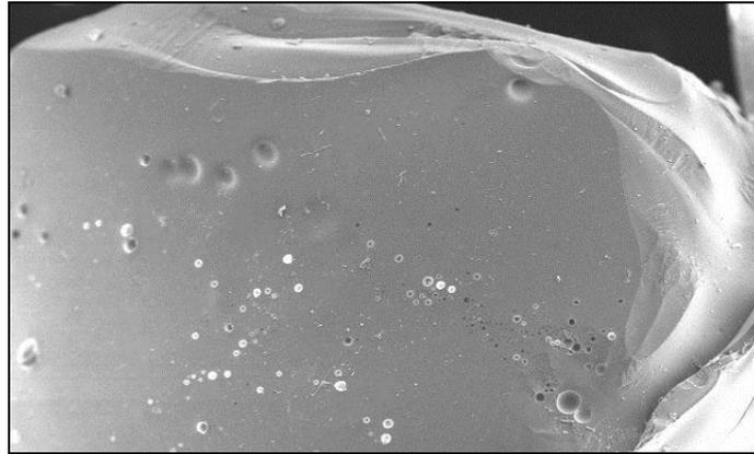
**Fig 4:** Structure of Low temperature water cooled slag
