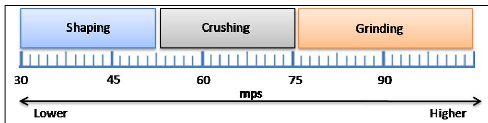
**Fig 6:** Effect of rotor velocity on particles in Vertical Shaft Impactor
