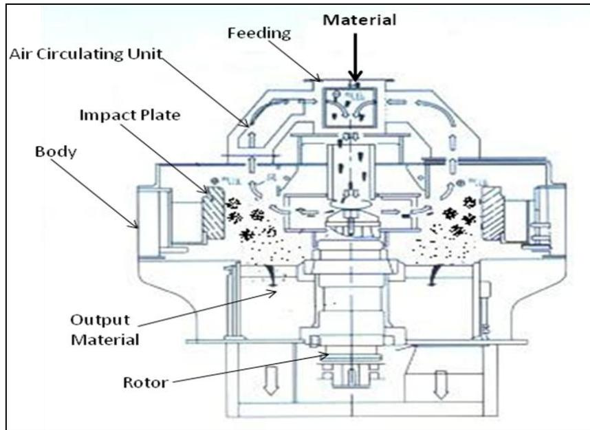
**Fig 5:** Vertical Shaft Impactor
