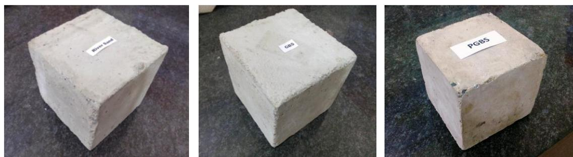
**Fig 9:** Concrete cubes made using river sand, GBS and PGBS
