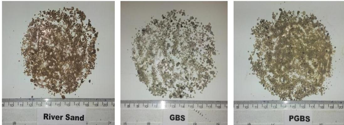
**Fig 7:** Particles of river sand, GBS and PGBS
