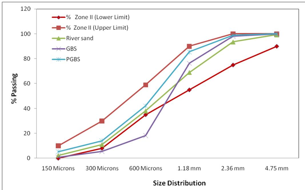
**Fig 8:** Size distribution curves of the GBS, PGBS and River sand
