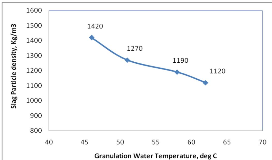
**Fig 3:** Effect of granulation water temperature on slag density
