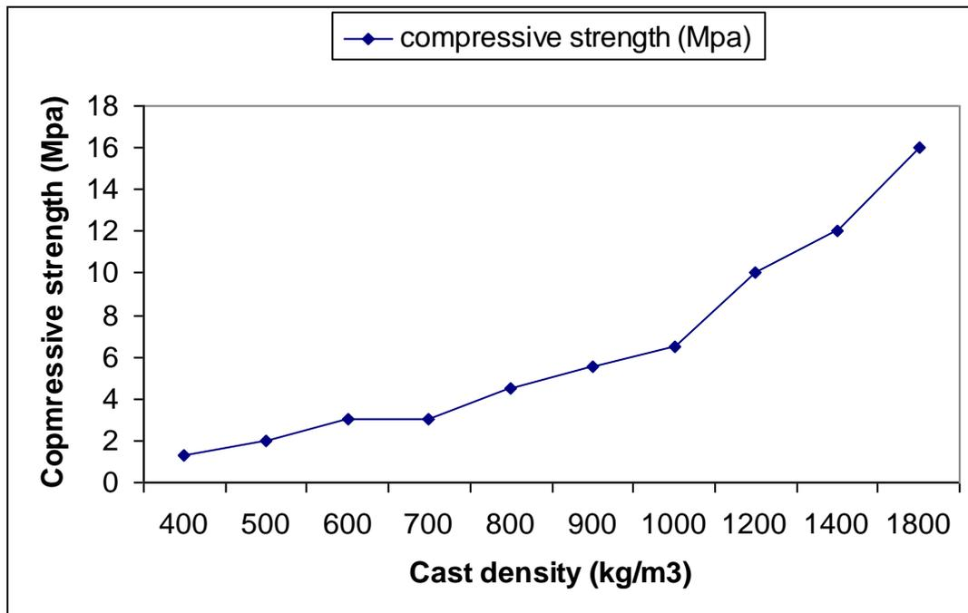
Fig.3 Relation between compressive strength and Cast density.
