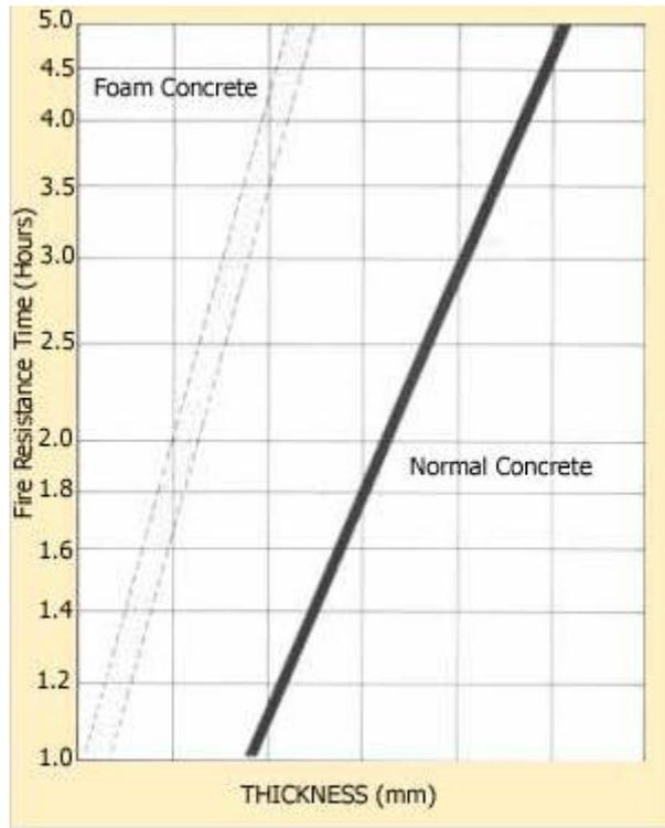
**Fig.4** Relation between fire resistance and thickness of foam concrete wall
