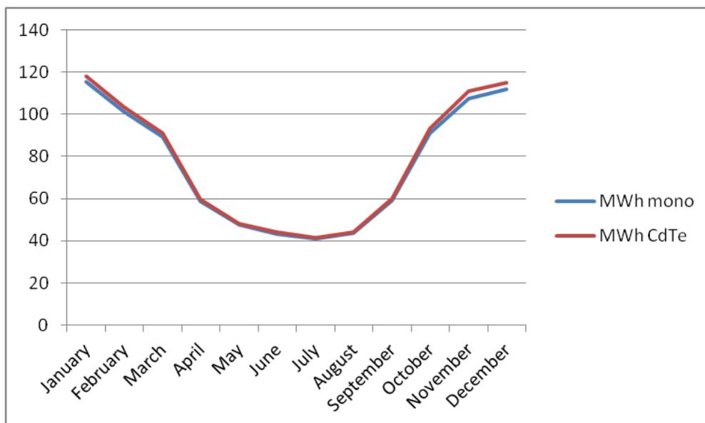
**Figure 7** - Monthly output variation for Solar PV Façade for Monocrystalline & CdTe with 90° tilt (vertical) in Mumbai, India[2]
