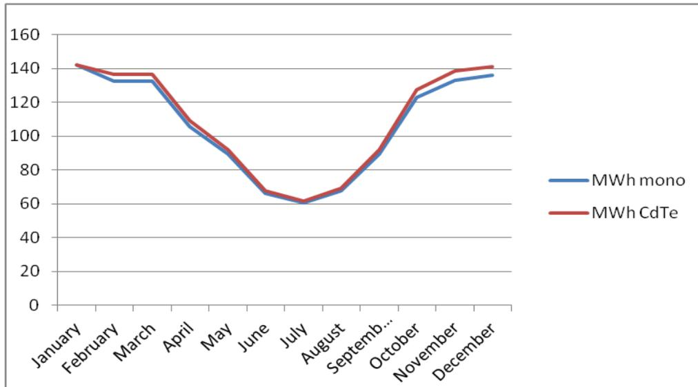
**Figure 6** - Monthly output variation for Solar PV Façade for Monocrystalline & CdTe with 65° tilt in Mumbai, India[2]
