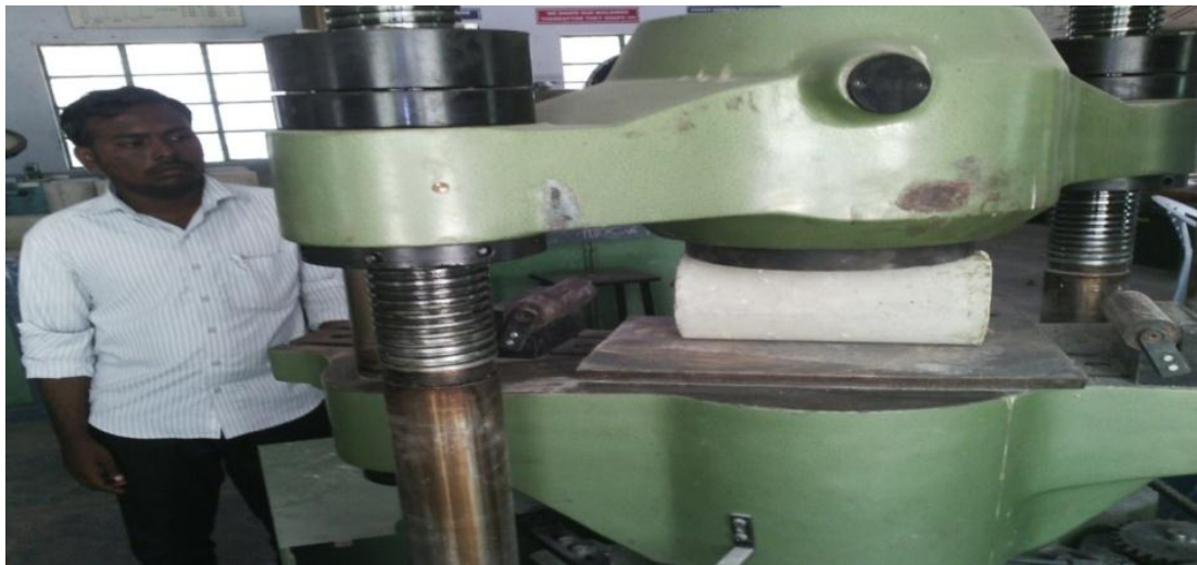
Figure 2 split tensile test on cylinders
