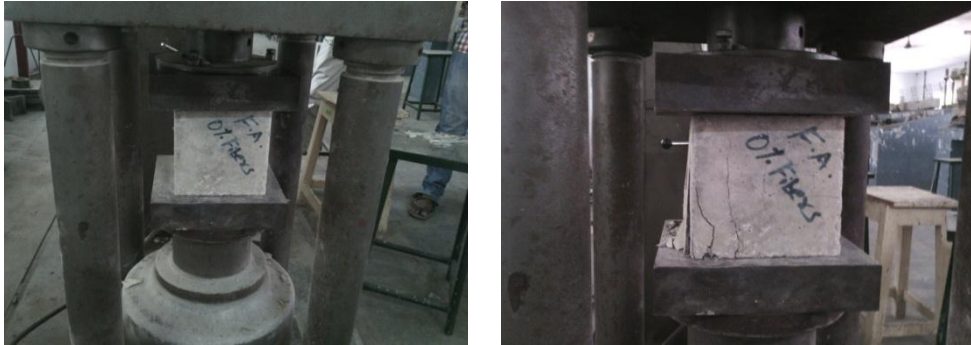
Figure1 compression test on cubes
