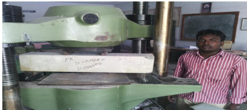
Figure3 flexural test on beams
